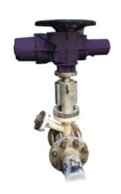
Piston Type Injection Valves have simplified paste batching plants and underground retic systems allowing plant operators to inject air and water for flushing and blockage control without the valve itself becoming a point of blockage in itself.
