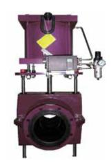
The PROEFILL Paste Batching Plant Hopper Outlet Control Valve's primary purpose is for flow control of paste out of the main hopper and into the gravity fed bore maintaining optimum feed velocity to prevent the segregation of solids and liquid.
