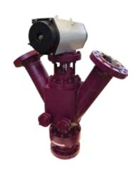
Primary purpose is for flow diversion of paste or tailings in both above ground and below ground reticulation systems, but can also be used in any high pressure abrasive slurry system to divert flow from one pipeline to another without costly and continual pipework disconnection and reconnection to change diversion of flow.
