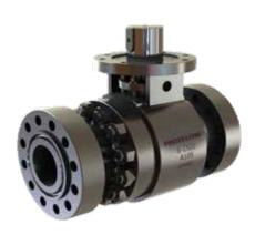
The PROEBALL provides in line isolation for high solids non cemented slurries, air injection isolation and high pressure water injection isolation in the harsh environment of paste batching plants and tailings distribution systems. These valves offer cost effective secondary isolation back-up within flush water injection systems with positive sealing against small fines found in process water supply.
